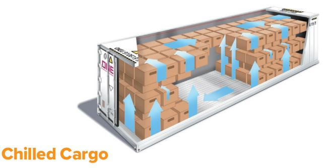
Chilled cargo is highly perishable premium food which can gradually ripen during shipment. In this illustration, the degree of air flow through the cargo is largely dependent upon the stuffing pattern at the door.
